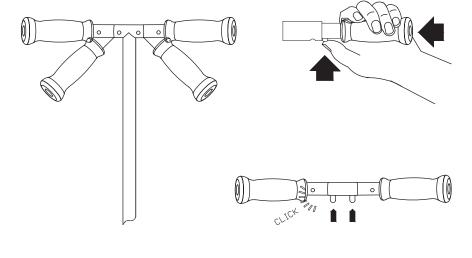
warning: Failure to properly engage the spring-loaded buttons may cause the handlebars to dislodge while riding and may cause you to lose control and fall. When correctly engaged, the handlebars will not rotate nor will they move sideways, and the spring-loaded buttons will be clearly visible in the holes on the T-Bar.
